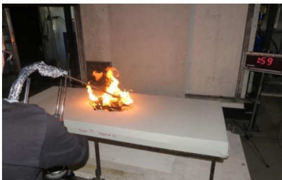
Photo 3 - Time 01:59. The burner is about to be removed.
