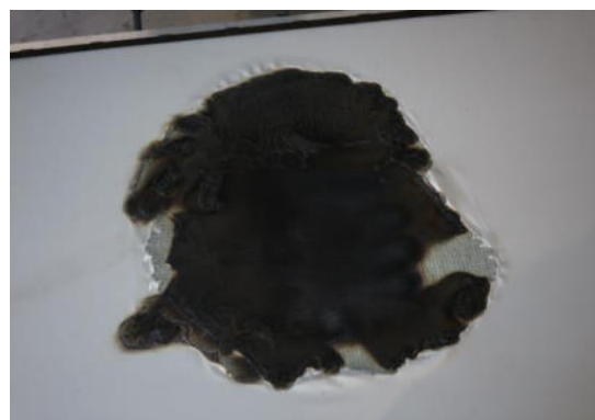
Photo 6 - Damage in the mattress after test.
