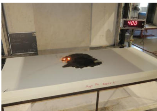
Photo 5 - Time 04:00. Most of the flames in the mattress have self-extinguished.
