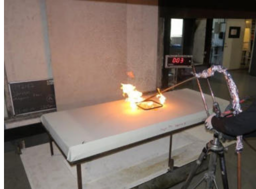
Photo 2 - Time 00:03. The burner has been applied.
