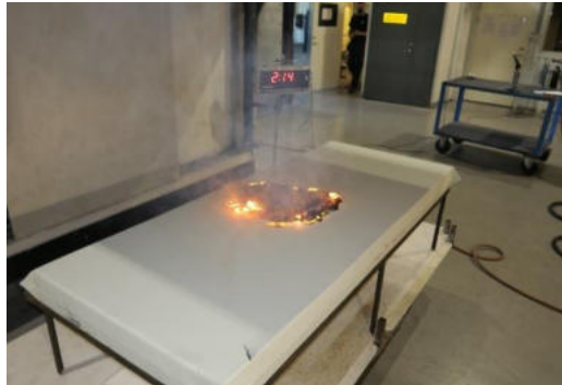
Photo 4 - Time 02:14. The mattress continues to burn at the edges of the burnt mattress cover.
