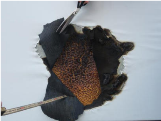
Photo 7 – Damage in the mattress after test.
