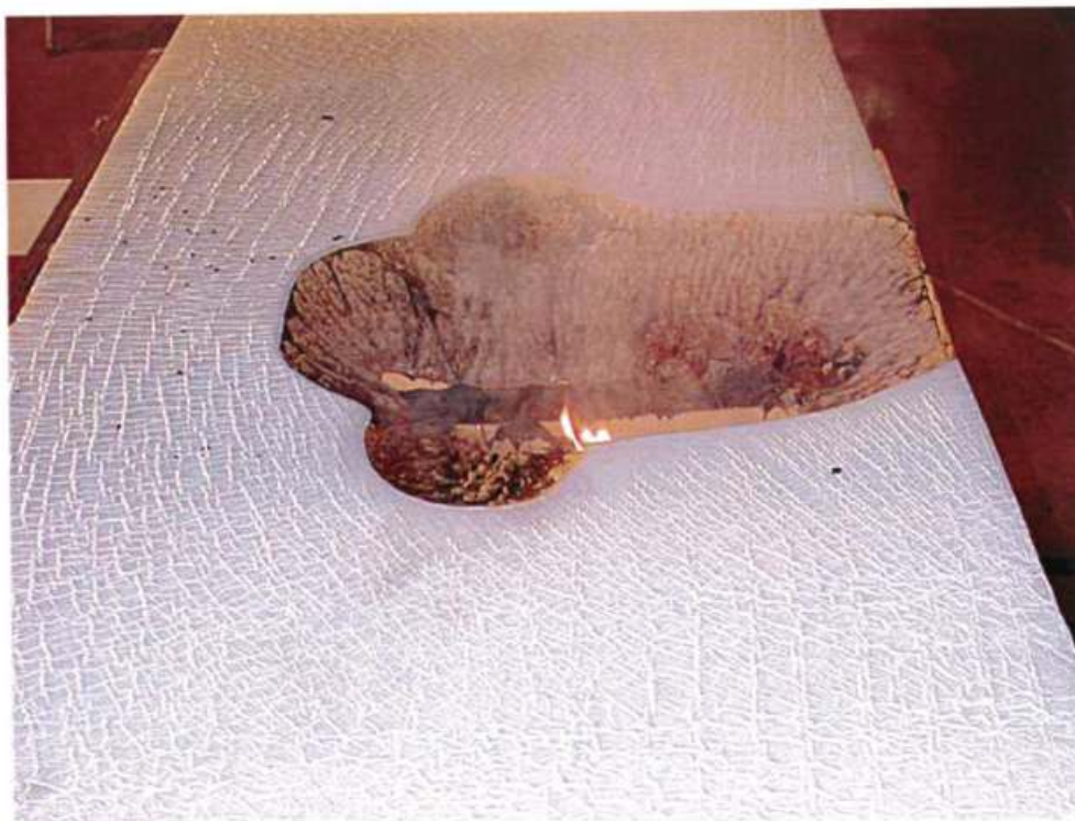
Photo no 10 Time 02:02 (min:s) Hygienbelagd madrass CMHR. Test 3. Limited flaming in the mattress.
