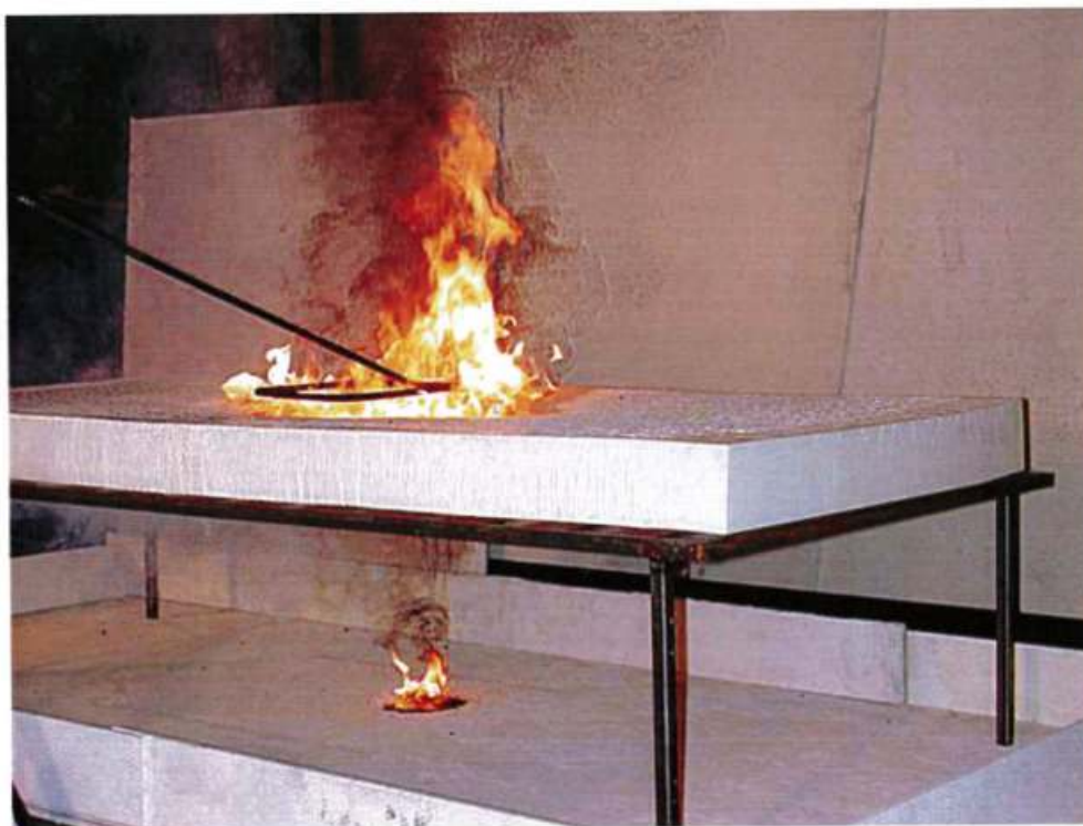
Photo no 8 Time 01:03 (min:s) Hygienbelagd madrass CMHR. Test 3. The melted material on the platform ignites.
