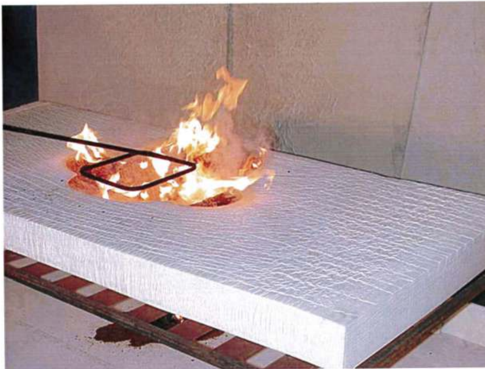
Photo no 9 Time 01:30 (min:s) Hygienbelagd madrass CMHR. Test 3. Heat release rate and smoke production rate decrease.
