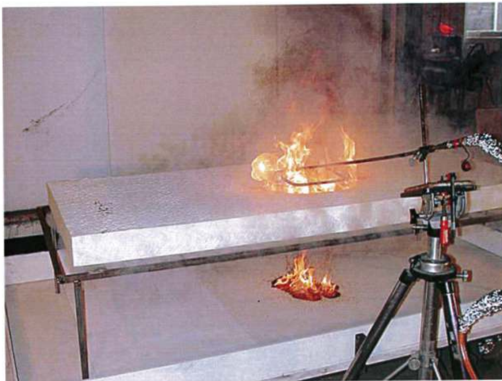
Photo no 3 Time 01:07 (min:s) Hygienbelagd madrass CMHR. Test 1. The melted material on the platform ignites.
