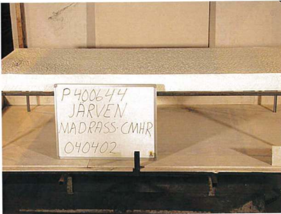
Photo no 1 Prior to test Hygienbelagd madrass CMHR. Test 1. The mattress is placed on a stand on the scale platform.
