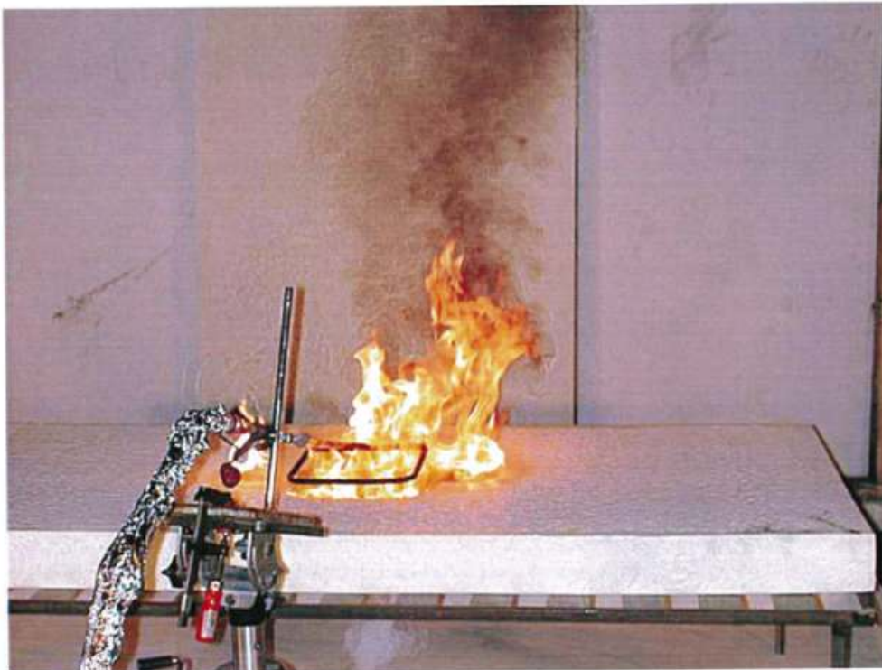
Photo no 2 Time 00:20 (min:s) Hygienbelagd madrass CMHR. Test 1. The cover and the foam core is ignited by the burner flames.
